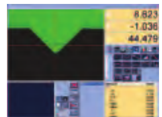
Pitch Slot Grinding with 3point Dresser
